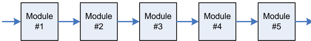
Figure 5. System containing only feedforward connections.
